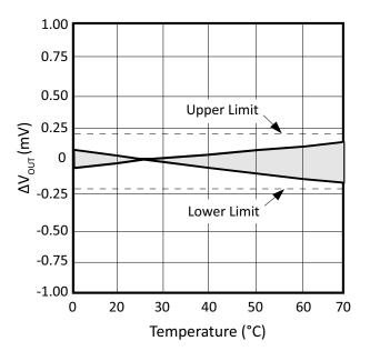
Figure 3: V<sub>OUT</sub> vs. Temperature (VRE305C)
